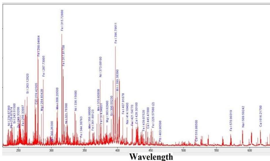
Fig 3.2 Illustrate LIBS emission spectra of the wavelength of the elements in the studied soil sample.
