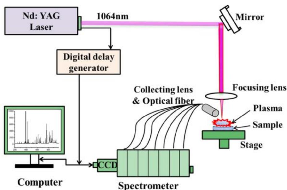
Figure 2.3. A schematic diagram of LIBS system [74].
