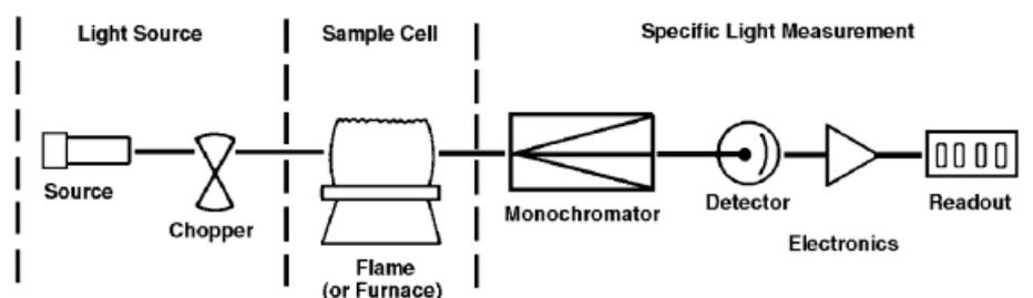
**Figure 2.1.** A schematic diagram of AAS system [38].
