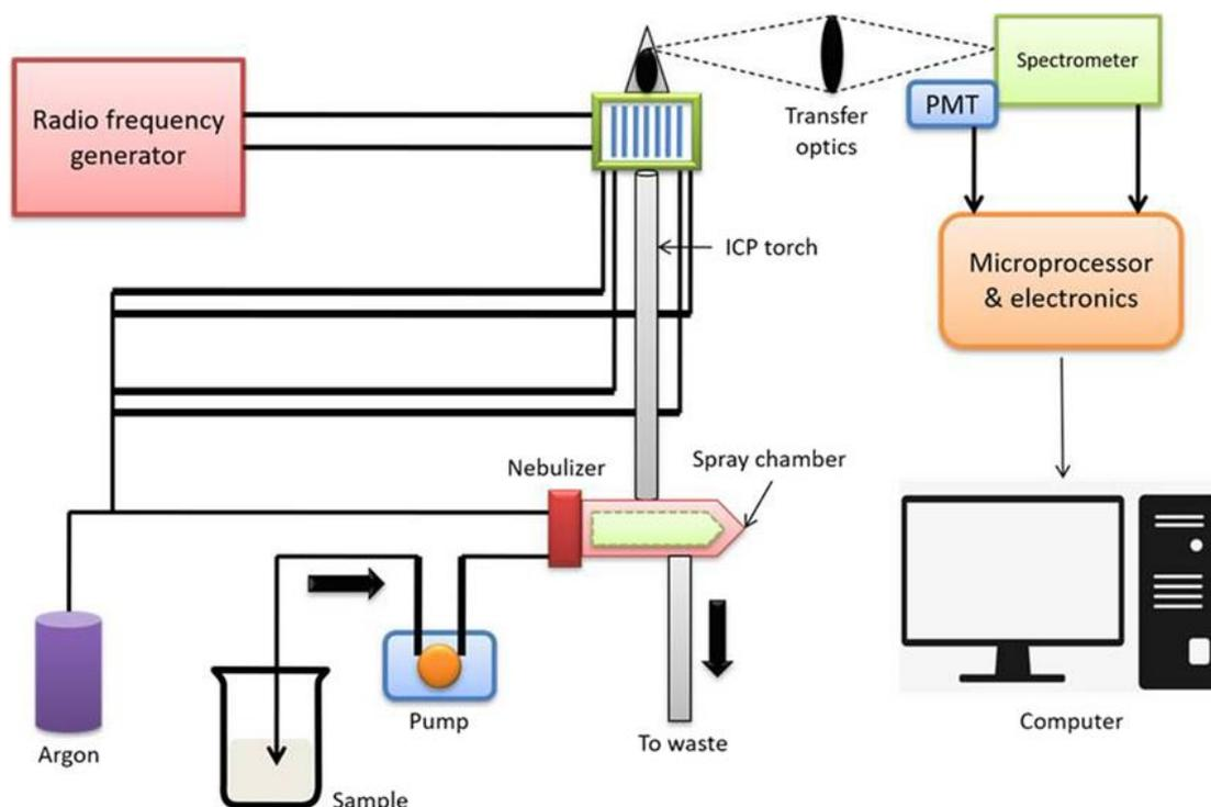
Figure 2.2. Instrumentation of ICP-OES [56].
